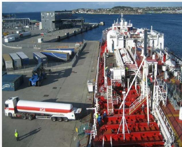
Tank truck to Ship Bunkering (TTS)
